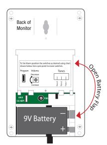
Note: Black ribbon goes underneath battery for easy removal.
